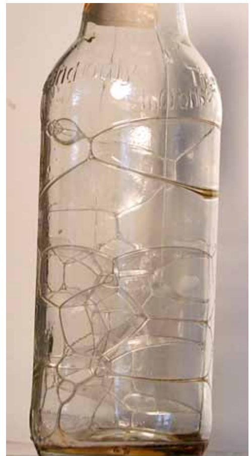
Figure 8.1(b) Beer bubbles model metal grains
