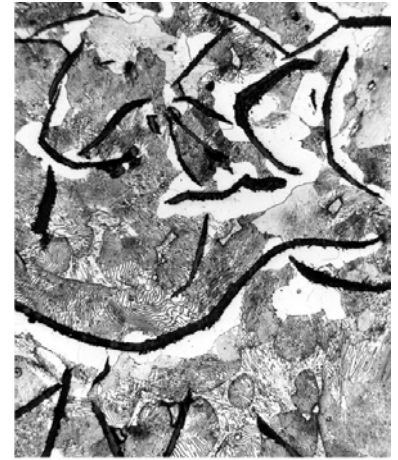
Figure 16.9 A gray iron with a ferrite-pearlite matrix. Mag. 250x.
